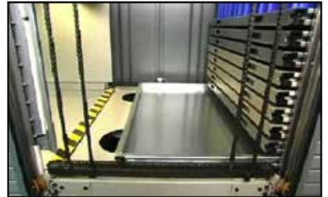
Chain is rigid for exact positioning, and provides a non-slip hold in an emergency stop.
